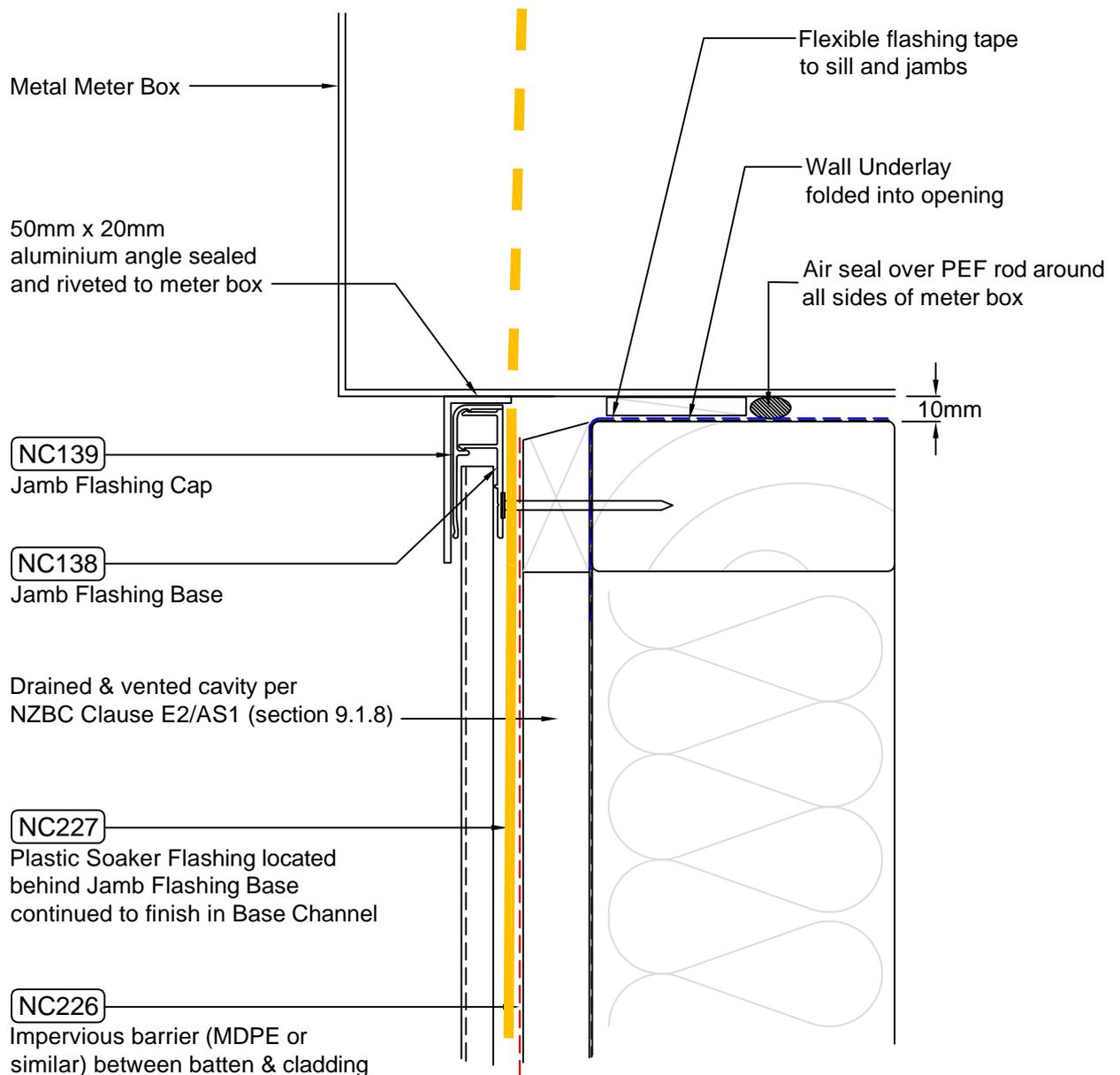
NW-V015C - Vertical Cladding over Drained & Vented Cavity - Meter Box Sill Detail
