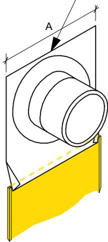
0.7mm Aluminium soaker flashing. Base tapered to fit in to plastic soaker flashing
