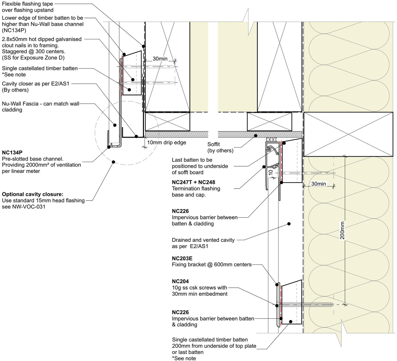
Flexible flashing tape over flashing upstand
